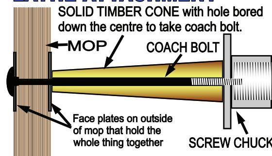
**BENCH GRINDER ATTACHMENT:** All mops come pre drilled and ready to use on a bench grinder that has a cone attached, it is simply a matter of screwing the buff onto a threaded cone. If you don't have one the cones, they are readily available at most hardware shops. You will need to remove the covers from the grinder to get full access to the mop and you may also want to remove the grinder wheel in order to get the most out of the buff.
